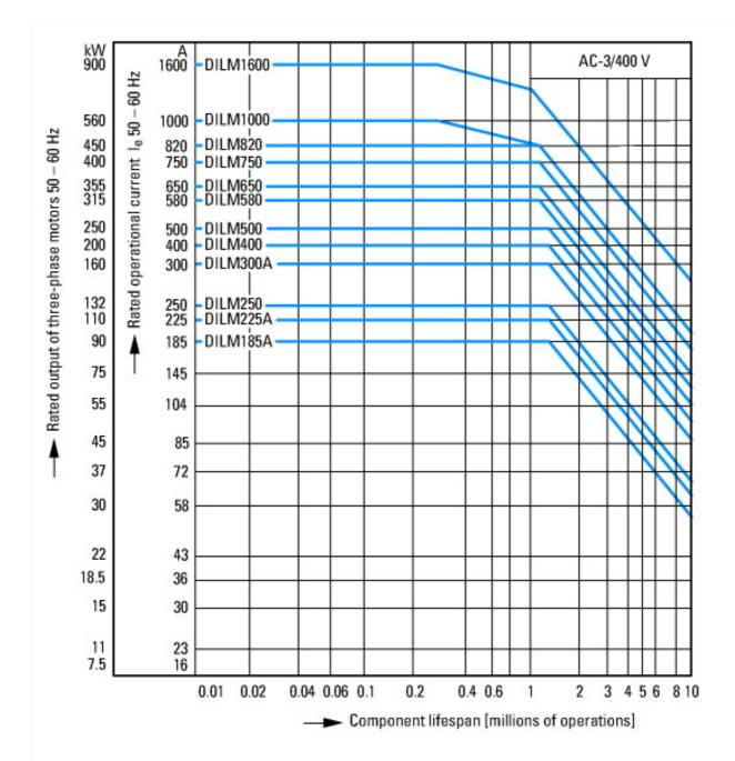
Normal switching duty Normal AC induction motor Operating characteristics Switch on: from stop Switch off: during run Electrical characteristics: Switch on: up to 6 x Rated motor current Switch off: up to 1 x Rated motor current Utility category 100 % AC-3 Typical Applications Compressors Lifts Mixers Pumps Escalators Agitators fan Conveyor belts Centrifuges Hinged flaps **Bucket-elevator** Air-conditioning systems General drives for manufacturing and processing machines
