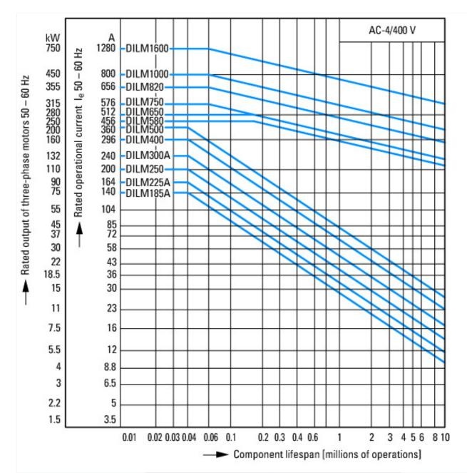
Extreme switching duty Squirrel-cage motor Operating characteristics Inching, plugging, reversing Electrical characteristics Make: up to 6 x rated motor current Break: up to 6 x rated motor current Utilization category 100 % AC-4 Typical applications Printing presses
