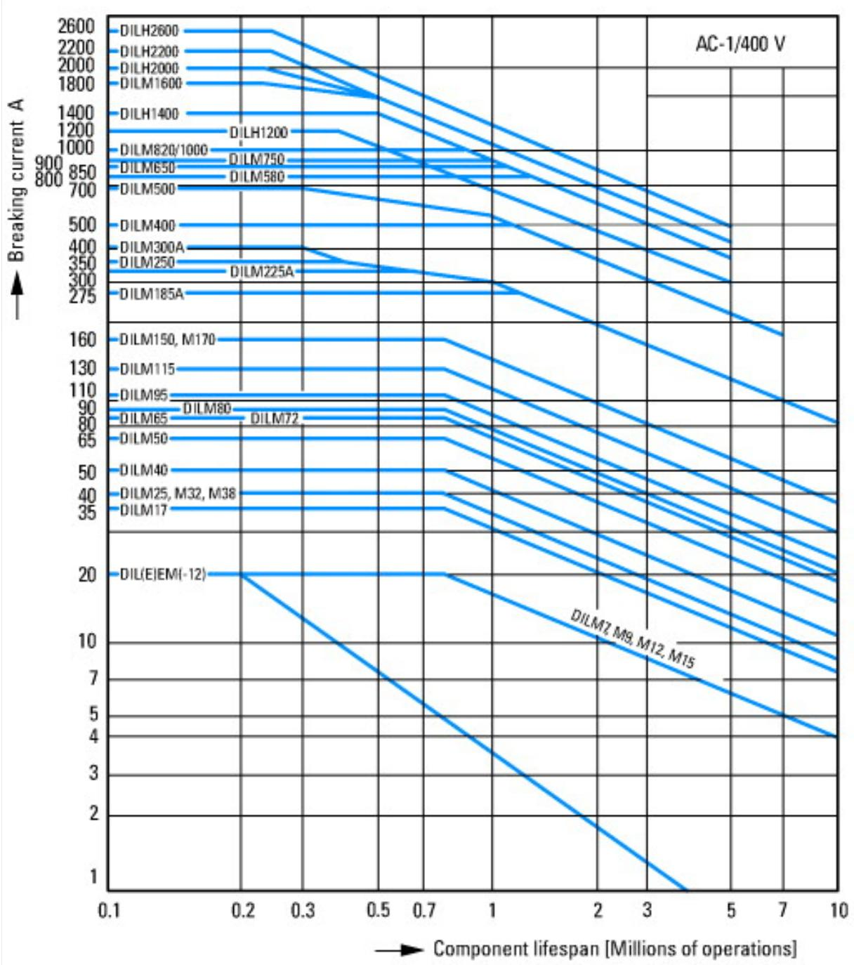
Switching conditions for 3 pole, non-motor loads
