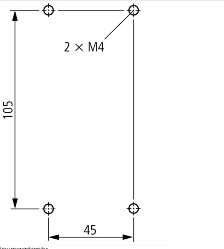
Lateral clearance to earthed parts: 6 mm
