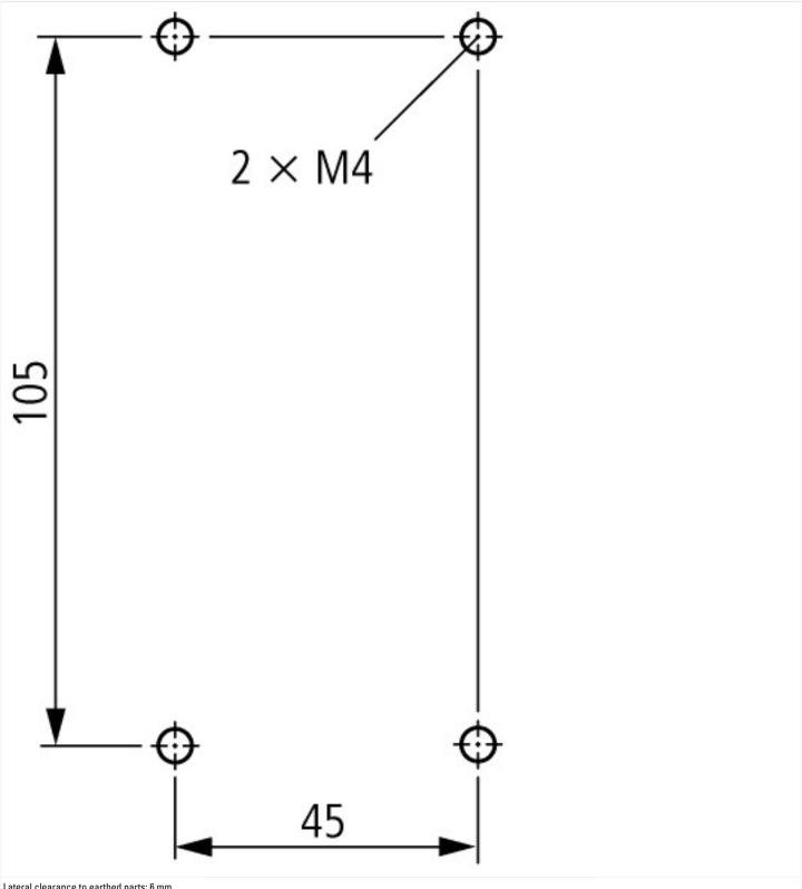
Lateral clearance to earthed parts: 6 mm
