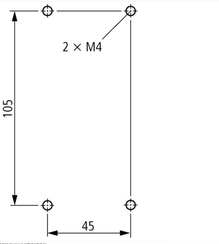
Lateral clearance to earthed parts: 6 mm
