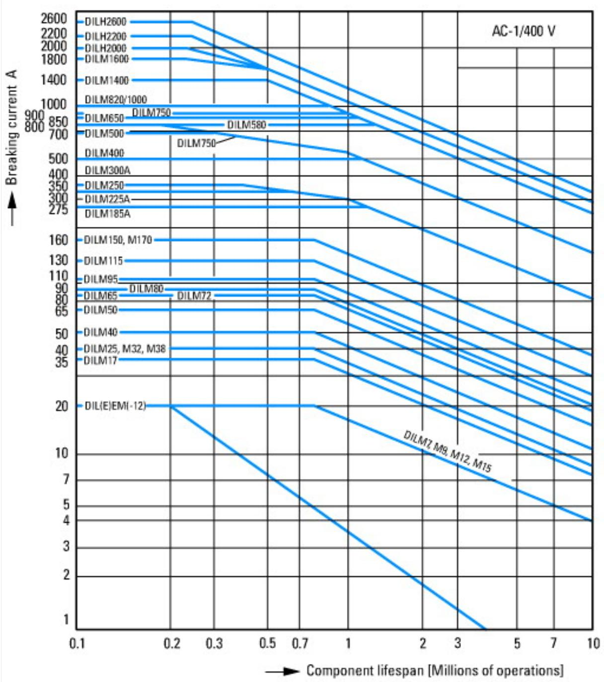
Switching duty for non-motor loads, 3-pole, 4-pole
