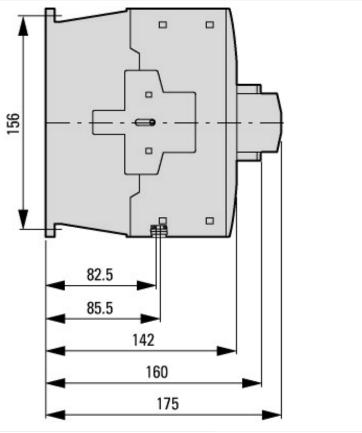
Contactor with auxiliary contact module
