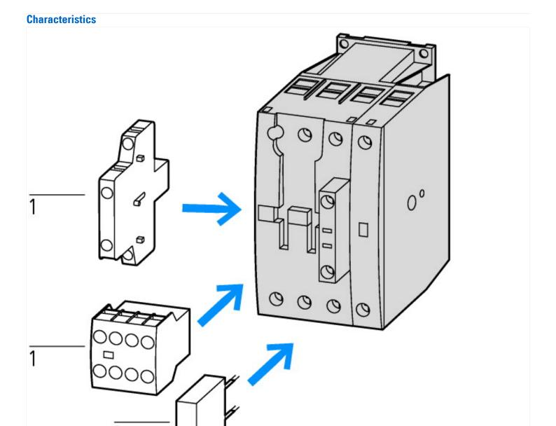
1: Auxiliary contact module 2: Suppressor
