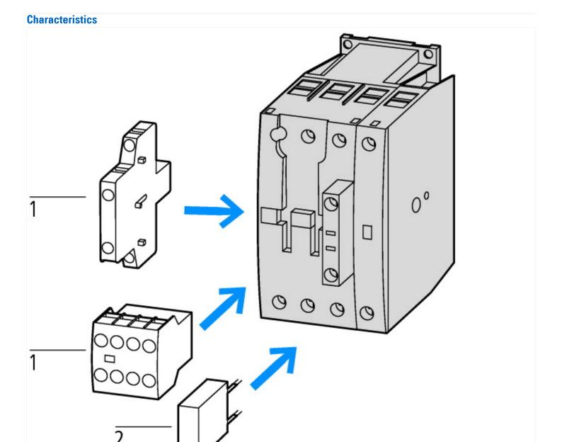
1: Auxiliary contact module 2: Suppressor
