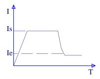
Fig2 Current Limit Startup Feature Curve
