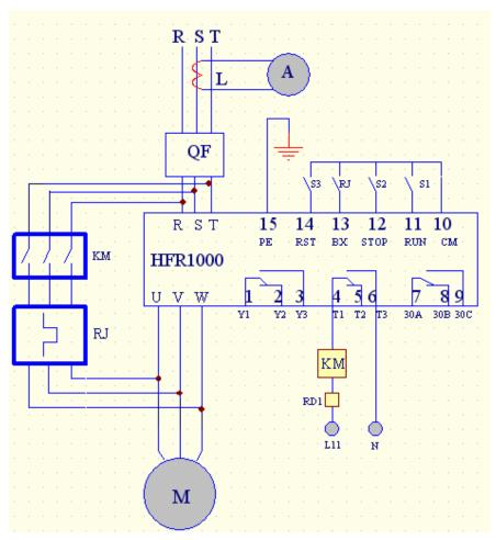
R, S, T terminals of softstarter are input terminals while U, V, W are output terminals. QF-auto air breaker, KM-contactor, RJ-over heating protection relay, RD1-fuse, L11—N is connected to 220V. And L11-N is forbidden being connecting to 380V.
