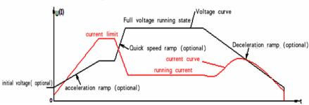
Soft Startup/Soft Stop Voltage (Current) Feature Curve
