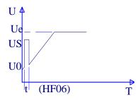
Fig3 Kick Startup Feature Curve
