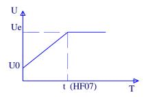
Fig1 Voltage Ramp Startup Feature Curve
