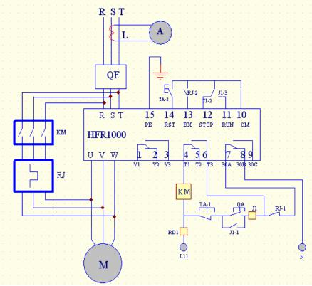
!PE Grounding wire should be as short as possible, and should be connected to the nearest grounding point, better on the installation board against the soft starter. Installation board should also be grounded.
