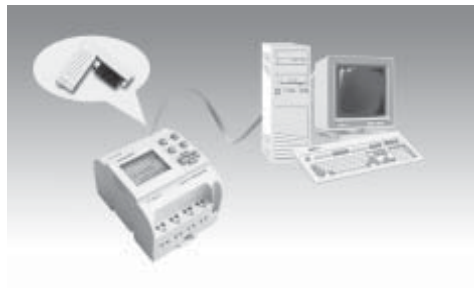
Fig. 4 . 24. FAB Communication Connection Frame
