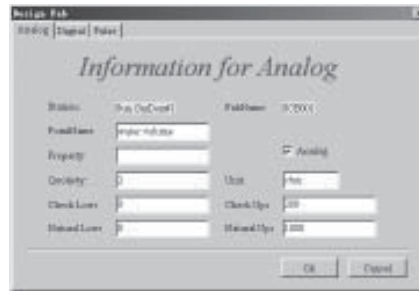
Fig. 4-14 Defining the Tele-metering Port
