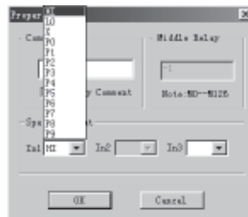
Fig. 3.16 Setting Properties for RS Relay
