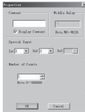
Fig. 3.15 Setting Properties for Blocks with Counters
