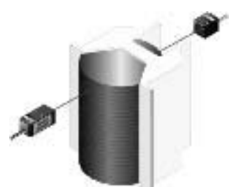
Sensing wafer position in wafer cassette
