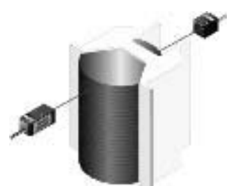
Sensing wafer position in wafer cassette
