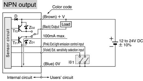
Symbols... D: Reverse supply polarity protection diode
