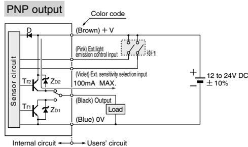
Symbols... D: Reverse supply polarity protection diode
