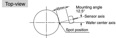
Note: If the wafer center axis and the sensor axis lie along a straight line, detection is not possible. Always mount the sensor at an angle to the wafer.
