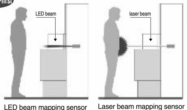
LED beam mapping sensor
