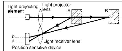
Fig. 1 Optical triangulation range measurement method
