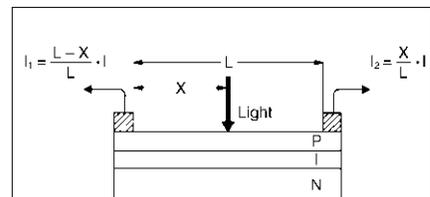
Fig. 4 PSD (position sensitive device) construction
