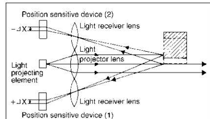
Fig. 2 Triple beam range measurement method
