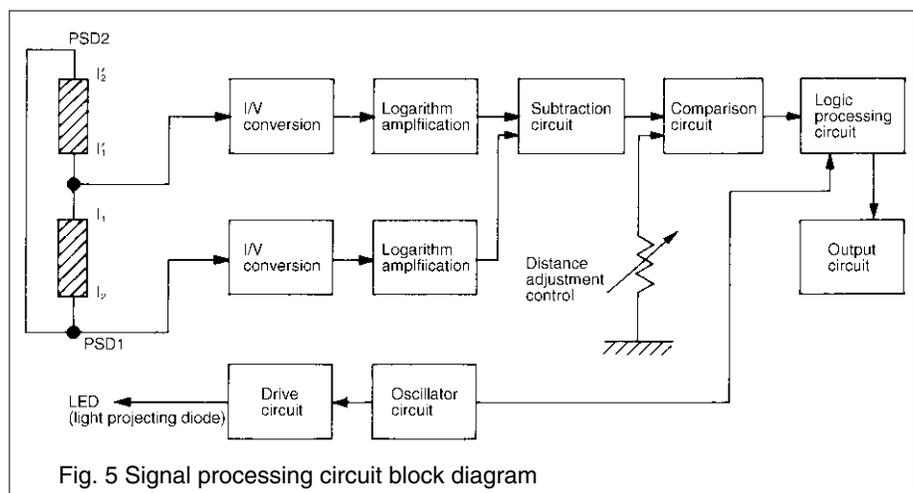
Fig. 5 Signal processing circuit block diagram
