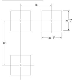
Note: The panel thickness should be 1 to 3.2mm.
