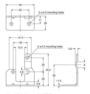
Material: Cold rolled carbon steel (SPCC) (Uni-chrome plated)
