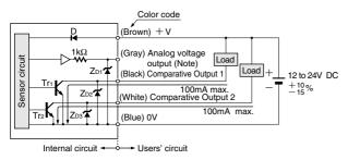
Note: When using the analog voltage output, take care to connect external device of proper input impedance. Also, when a cable extension is used, voltage drop due to cable resistance should be taken into account.
