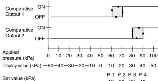
Note: As in the case of the hysteresis mode, the displayed values and the ON/OFF points of the output are shifted also in case the output mode is set to the window comparator mode.
