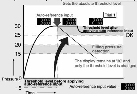
When auto-reference input is applied, the reference pressure '30' is added to the threshold level. If the reference pressure changes to '20' or '40', the auto-reference input compensates for this every time by changing the threshold level, so any variation in the filling pressure can be ignored.
