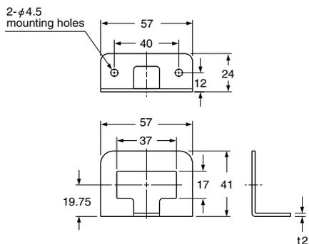
Material: Cold rolled carbon steel (SPCC)
