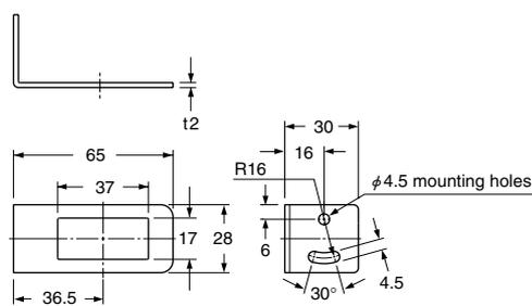
Material: Cold rolled carbon steel (SPCC)
