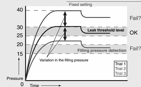
Because the threshold is fixed for conventional pressure sensors, changes in the reference pressure result in wrong decisions.
