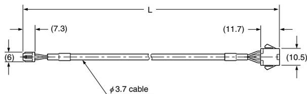
Note: The heat-shrink tube for the standard cable is black, and the heat-shrink tube for the flexible cable is gray.
