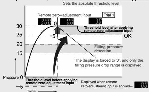
When remote zero-adjustment input is applied, the reference pressure is forced to '0'. If the reference pressure changes to '20' or '40', the remote zero-adjustment input adjusts the reference pressure to '0' every time the reference pressure changes, so any variation in the filling pressure can be ignored.
