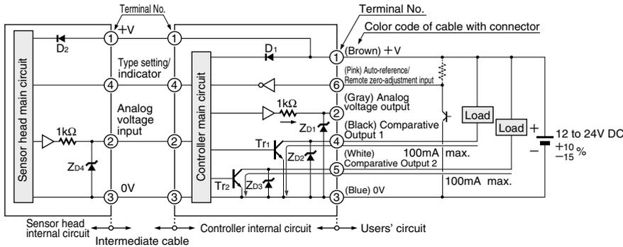
Symbols... D<sub>1</sub>, D<sub>2</sub>: Reverse supply polarity protection diode
