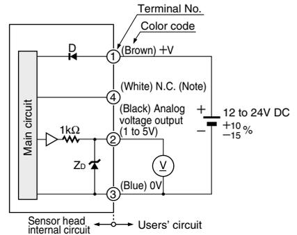
Note: In case the pressure sensor head is used independently, insulate the white wire (Terminal No.4) and keep it open.
