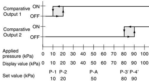
Note: As in the case of the hysteresis mode, Set Value P-3 and Set Value P-4 are shifted also in case the output is set to the window comparator mode or the leak test mode.
