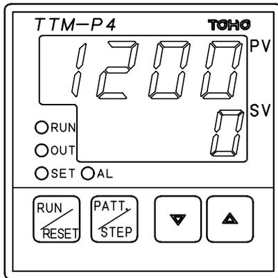
PV: Displays the temperature measured.
