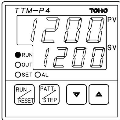
PV: Displays the temperature measured.
