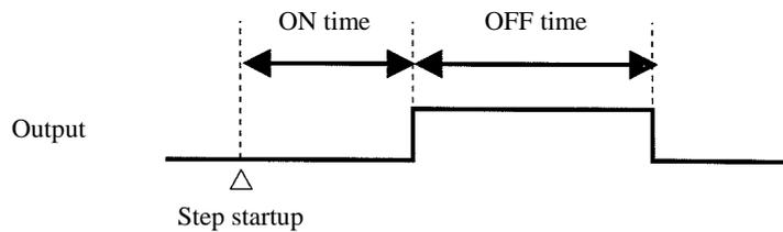
\* The time signal output will be shared with an alarm output, so that it will be invalid when an alarm output is selected.
