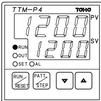
PV: Displays the temperature measured.
