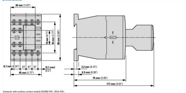
Contactor with auxiliary contact module DILA-XHIT...
