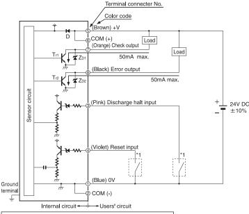
Symbols... D: Reverse supply polarity protection diode ZD1, ZD2: Surge absorption zener diode Tr1, Tr2: NPN output transistor
