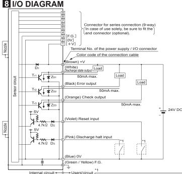
Z<sub>D1</sub>, Z<sub>D2</sub>, Z<sub>D3</sub>: Surge absorption zener diode Tr<sub>1</sub>, Tr<sub>2</sub>, Tr<sub>3</sub>: NPN output transistor
