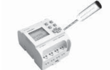
Fig. 2.1 Remove LCD panel as instructed
